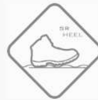
Slip Resistance Heel (Forward) Coefficient of Friction: \geq 0.31 (ceramic & Cleaner) \geq 0.19 (Ceramic & Glycerin)
