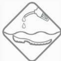
Hydrocarbon Outsole Fuel Oil Resist Volume Increase \leq 12\%
